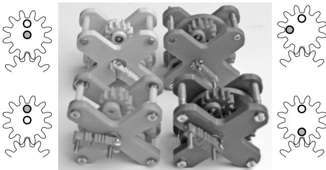
Fig. 6: Proof-of-concept prototype Orbitless drives
